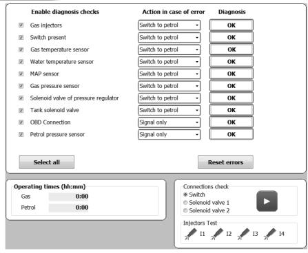
When the GAS control unit detects a diagnosis error on the parameter read, takes the action selected in the "Action in case of error" corresponding to the error detected.
