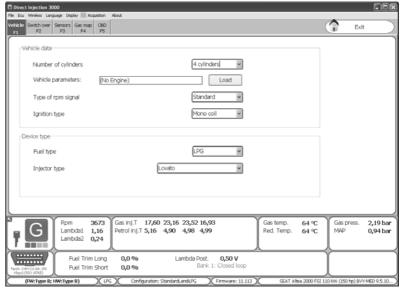
In the part underneath all of the pages, a display summarising the current values of the general system operation signals is provided.
