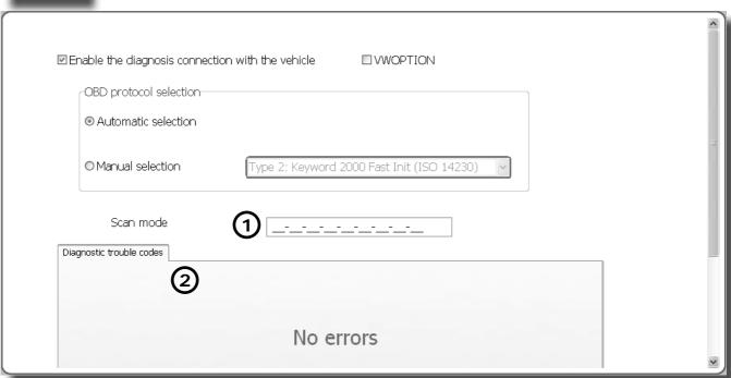
Enabling the diagnostic OBD connection ( $\boxed{\mathbf{V}}$ ) the user can select the control unit connection mode to the OBD protocol:
